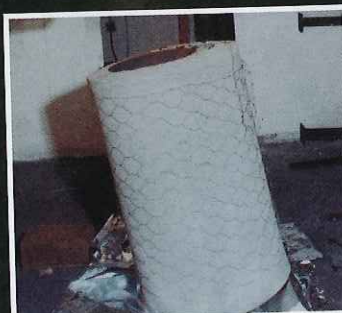
CR SAFGUARD fire resistant mattress foam (ASTM F1085 Annex 3 at 3 1/2 minutes)
